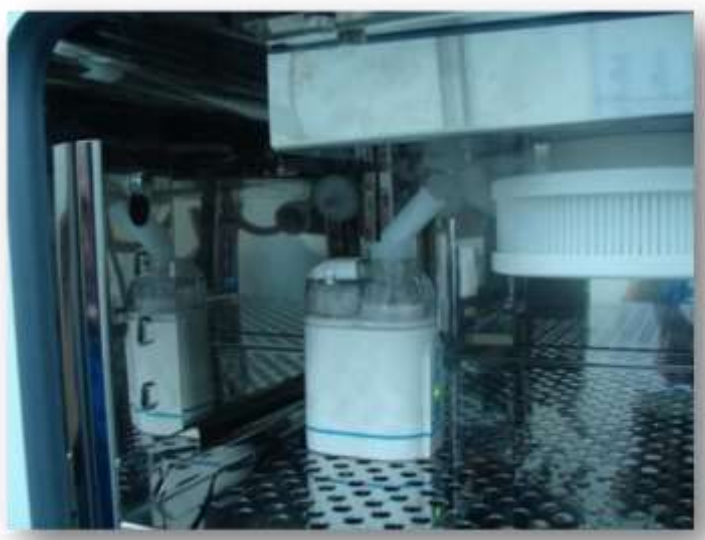
Figure 1. Smoke test to check the airflow pattern
